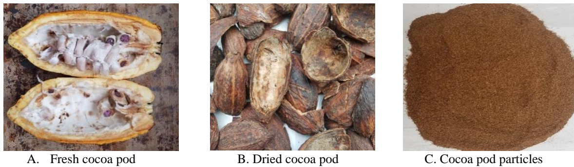
Fig. 3 Stages of processing of Theobroma cacao pod into particles
