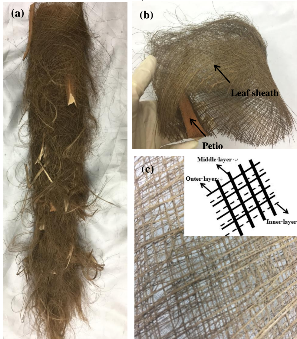
Figure 1 Photograph of (a) windmill palm tree covered with leaf sheath; (b) leaf sheath; (c) a small piece of leaf sheath showing the arrangements of different layers of fiber bundle, with inserted images showing the schematic view of fiber arrangement.
