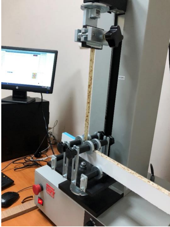
Figure 2.a. PB edge banding test started
