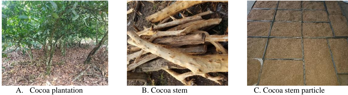
Fig. 2 Stages of processing of Theobroma cacao stem into particles
