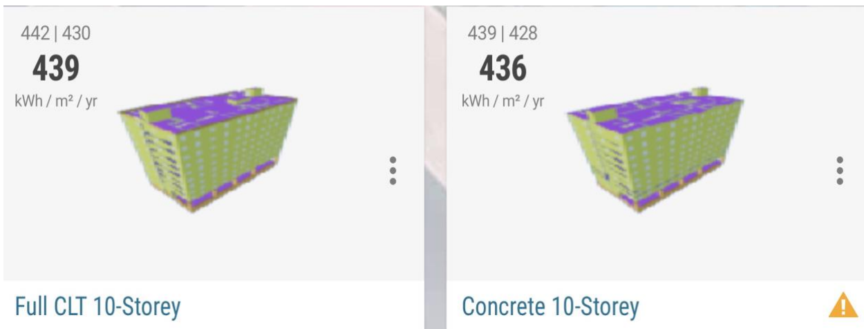
Figure 6. Energy use intensity simulation of the 2 alternatives of the 10-storey building
