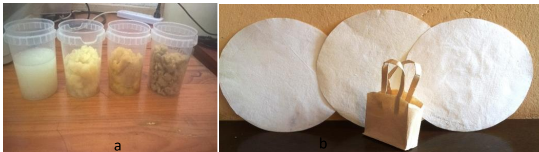
Figure 1. (a) Brightness changes during bleaching, (b) Paper hand sheets fabricated from thatching grass fibers, and a shopping bag.
