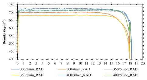
Fig. 3: Density profiles of specimens one-sided carbonized 300/350 and 400°C
