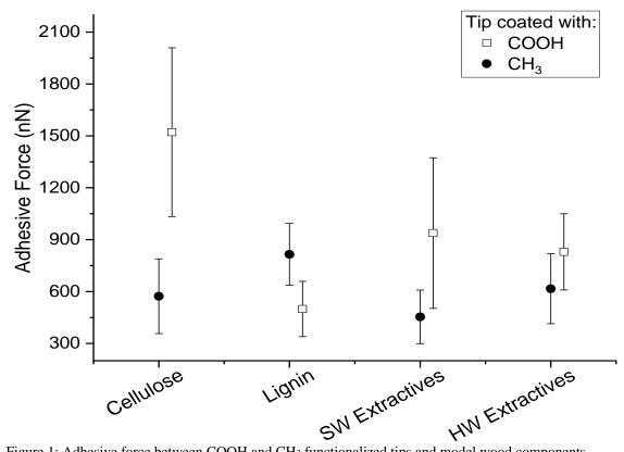
Figure 1: Adhesive force between COOH and CH3 functionalized tips and model wood components
