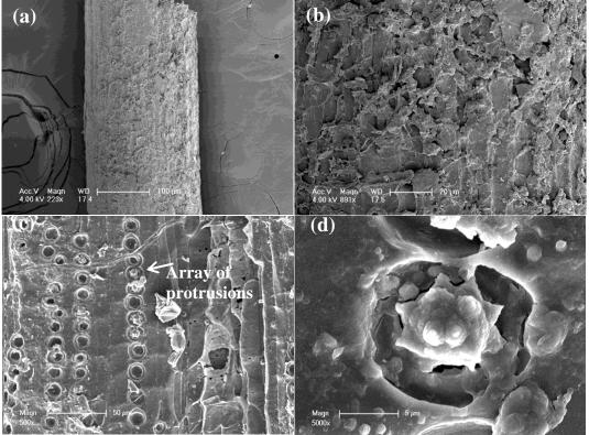
Figure 3 Surface morphological characterizations of palm fibers in outer layer: (a) sub-cylindrical shape, (b) waxy and course surface, (c) arrays of protrusions embedded with (d) silica.
