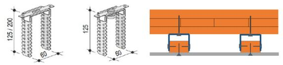
Figure 1. Hangers for wall (and ceiling) mounting of wooden slats with and without resilient layers under the mounting screw and a schematic view of the investigated building element made of CLT slab with hangers, wooden slats and plasterboard.
