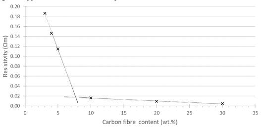
Figure 11: P1 - resistivity over carbon fibre content of panel nr. 2 to 7 manufactured with CF1.
