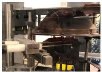
Figure 2: A picture of the cone calorimeter
