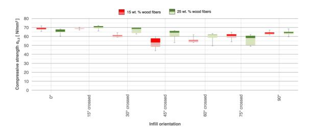
Figure 4: The behavior of the compressive strength  $\sigma_{0,2}$  depending on the infill orientation (infill pattern) applied and the fiber content (composite #1 or composite #2) in the wood/PLA composite.
