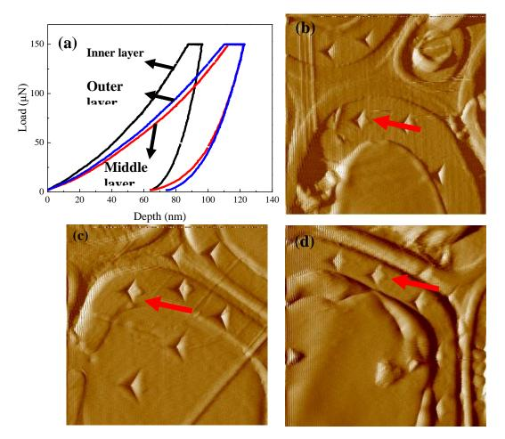
Figure 5 (a) Typical load-depth curves of nanoindentation tests in cell wall of windmill palm fibers in different layers; Residual indentations on cell wall of windmill palm fibers in (a) inner, (b) middle, (c) outer layer.
