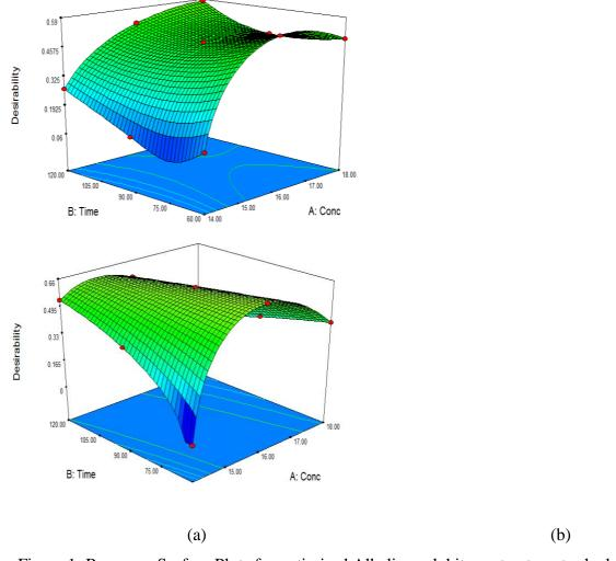
Figure 1: Response Surface Plots for optimised Alkaline sulphite pretreatment schedule for (a) WS (b) RF.
