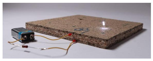
Figure 10: Conceptual testing of the conductive particle board connected to the pin with an LED and a battery.
