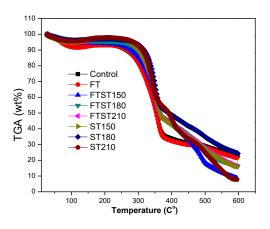
Figure 5: TGA curves of control and two-step freeze-silicone treated Masson Pine wood.
