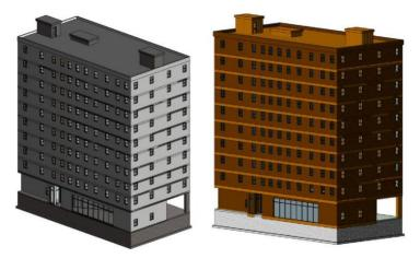
Figure 3. Two alternatives for design: Concrete (left) and CLT (right).
