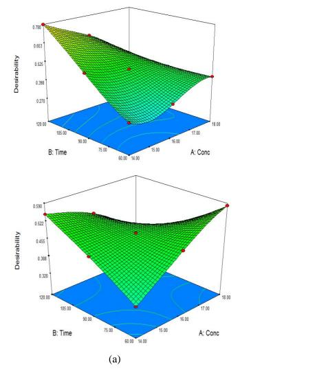
Figure 2: Response Surface Plots for optimised NaOH pretreatment schedule for (a) WS (b) RF. CONCLUSION
