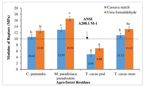
Fig. 7 Modulus of rupture of particleboards produced from agro-forest residues
