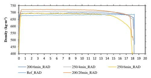
Fig. 2: Density profiles of reference and one-sided specimens carbonized at 200/250°C
