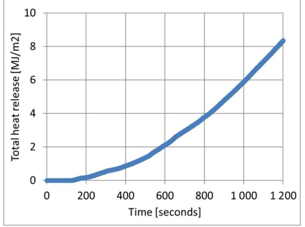
Figure 3: The total heat release according to ISO 5660 illustrated cumulatively. The determinative value of 8 MJ/m<sup>2</sup> is reached after 1172 seconds.
