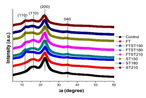
Figure 3: X-ray diffraction pattern of control and treated Masson Pine wood using two-step freeze-silicone oil treatment.
