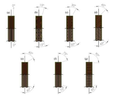
Figure 1: All seven infill patterns applied for fabricating the test specimens  $|(a) 0^{\circ}|(b) 15^{\circ}$  crossed  $|(c) 30^{\circ}$  crossed  $|(d) 45^{\circ}$  crossed  $|(e) 60^{\circ}$  crossed  $|(g) 90^{\circ}$
