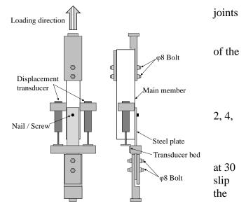
Fig.5. Outline of the shear tests.
