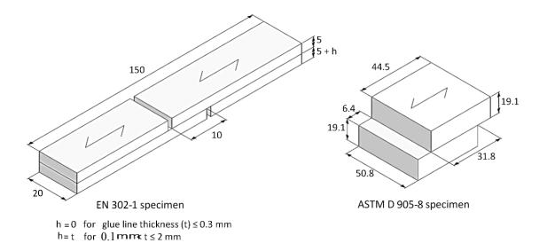
Figure 3. Configurations of EN 302-1 and ASTM D 905-8 specimens. Measurements in mm.
