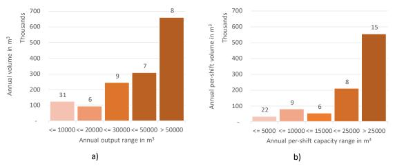
Figure 5: Annual production volumes (a) and annual per-shift capacity (b) allocated to CLT lines representing a range of production capacity scale. Number of production lines in each category provided above the bars.
