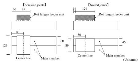
Fig.4. Outline of decay treatment using rot fungus feeder units.
