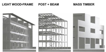
Figure. 2. Three wood building construction systems (WW-WSP 12)
