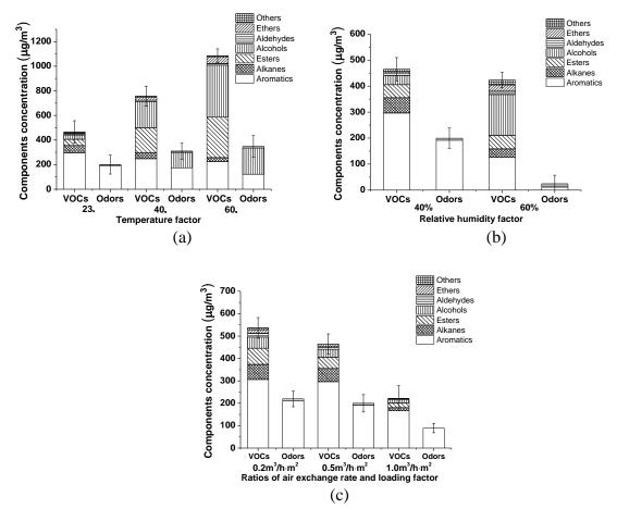
**Figure 6.** TVOCs and odor components concentrations from veneered particleboard coated with water-based lacquer under different conditions at an equilibrium state: (a) different temperatures; (b) different relative humidity values; and (c) different air exchange rate to loading factor ratios.
