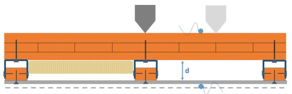
Figure 3. Schematic mock up wall element with 100 mm CLT slab and variation of 1 or 2 plasterboards, type of plasterboard, type of hanger, cavity filling and distance d between the coupled masses.
