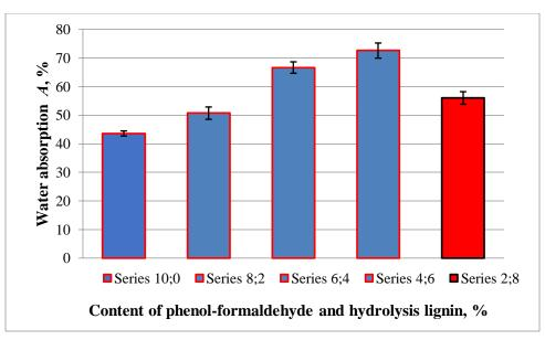
Figure 1. Water absorption of dry-processed fibreboards at various content of phenol-formaldehyde resin and hydrolysis lignin
