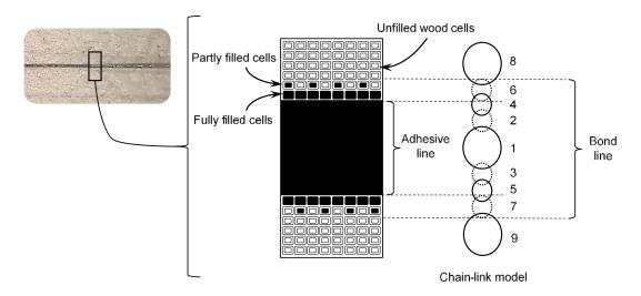
Figure 1. Illustration of the chain-link model in a wood-wood glued element.
