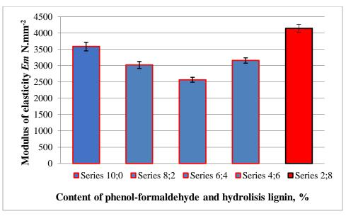
Figure 4. Modulus of elasticity of dry-processed fibreboards at various content of phenol-formaldehyde resin and hydrolysis lignin
