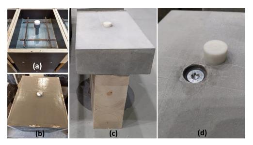
Figure 3. A T-section glulam-concrete deconstructable connection. (a): the prepared formwork, (b): concrete cast onto the formwork, (c): the resulting T-section connection, and (d): the screw head inside the connector after removing the rubber lid.
