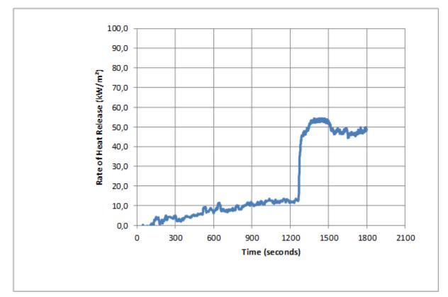
Figure 4: The heat release rate over the observation according to ISO 5660. The threshold value of 200 kW/m<sub>2</sub> is never reached.
