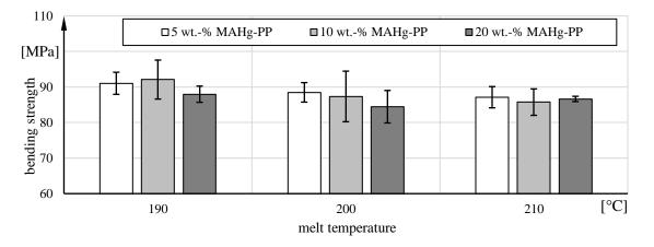
Figure 4 Dependence of bending strength on melt temperature and bonding agent content
