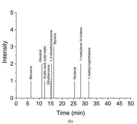
Figure 3. Gas chromatography (GC) total ion flow chart and odor-time intensity spectrum: (a) water paint coating particleboard, (b) particleboard.
