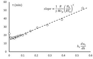
Figure 2. Plot of the experimental effective response time constant  $\tau$  (Eqn. (9)) versus  $h_1(du_1/dh)$ , confirming TLMT behavior (Eqn. (7)). The broken line is a linear regression fit for the data points > 0.05 (abscissa).
