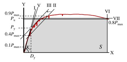
Fig.7. Method of evaluating shear performance of the joints.  $K_s$ , initial stiffness;  $P_{max}$ , maximum shear resistance;  $P_y$ , yield shear resistance;  $D_y$ , yield displacement;  $P_u$ , ultimate shear resistance.
