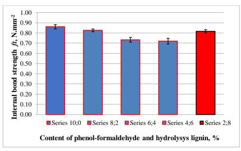
Figure 5. Internal bond strength of dry-processed fibreboards at various content of phenol-formaldehyde resin and hydrolysis lignin
