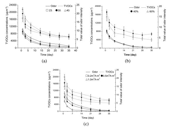
Figure 5. TVOCs concentration and total odor intensity of the water-based lacquer veneer particleboard at (a) different temperatures, (b) different relative humidity values, and (c) different air exchange rate to loading factor ratios.
