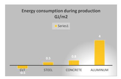
Figure. 1. Energy consumption during production in GJ/m2
