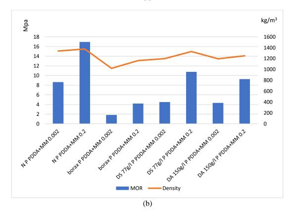
Fig.3: MOR and Density of CBPB made of poplar. (a) boards made with water glass additive, (b) boards made with PDDA+ montmorillonite additive
