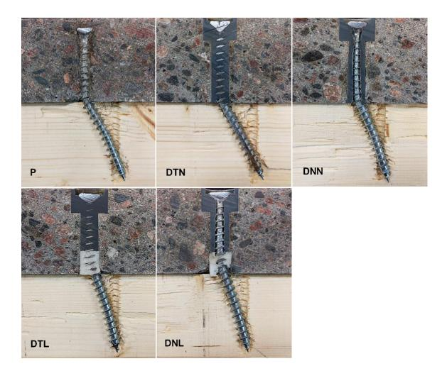
Figure 6. Failure modes of the test connections.
