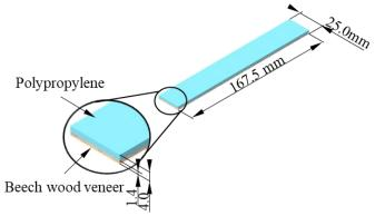
Figure 3 Polypropylene-wood veneer bending specimen
