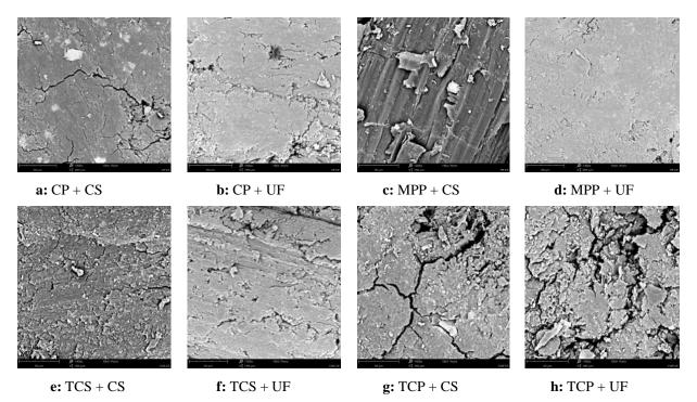
**Figure 9**: Figures 9a to 9f show smooth surfaces indicating good compatibility between particles and adhesives. Figures 9g and 9h show discontinuity of particles and adhesives, thus detached particles from adhesives surfaces. **Legend:**  $CP = Ceiba \ pentandra$ :  $MPP = Musa \ paradisiaca \ pseudostem$ :  $TCP = Theobroma \ cacao \ pod$ :  $TCS = Theobroma \ cacao \ pod$ :  $TCS = Theobroma \ cacao \ starch$ :  $UF = Urea \ formaldehyde$
