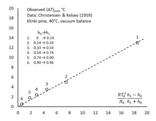
Figure 1. Verification of Equation (8) for the TLMT-predicted RH-trend of  $(\Delta T)_{\text{peak}}$  for various humidity steps  $h_0 \rightarrow h_1$  (abscissa) versus the observed peak temperature (ordinate).
