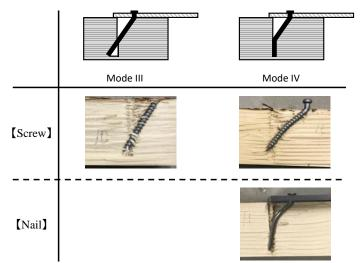
Fig.6. Observed failure modes of the specimens.
