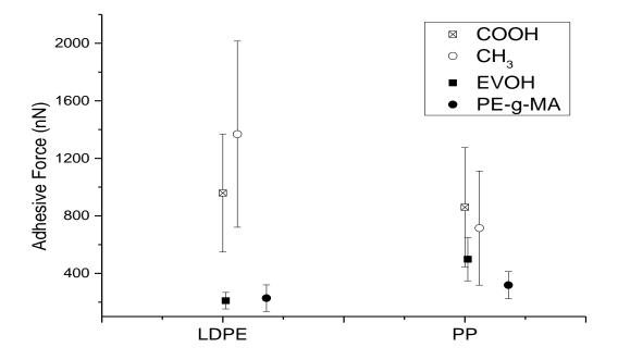
Figure 3: Adhesive force between different functionalized tips and model wood components
