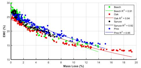
Figure 1. Exponential correlation between equilibrium moisture content (EMC) at 20°C and 99% relative humidity (RH) and mass loss of various thermally modified wood species
