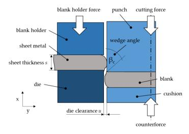
Figure 1 Basic terms of shear cutting process
