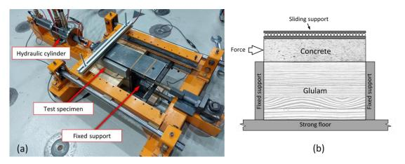
Figure 4. (a) The push-out test set-up used and (b) the side-view of a specimen under loading.
