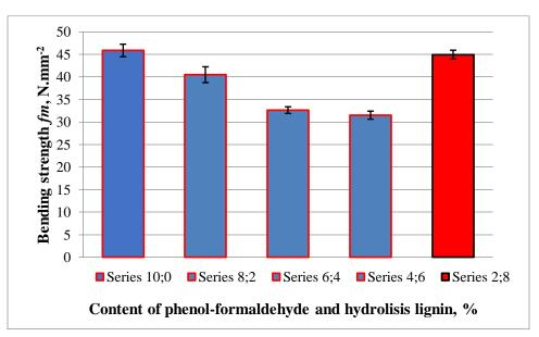
Figure 3. Bending strength of dry-processed fibreboards at various content of phenol-formaldehyde resin and hydrolysis lignin
