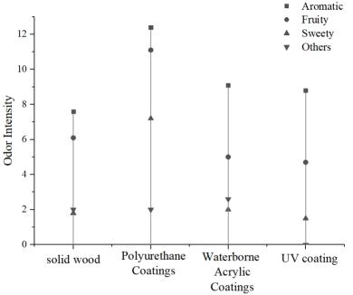
Figure 2 Relation diagram of odor concentration and odor intensity of four boards
