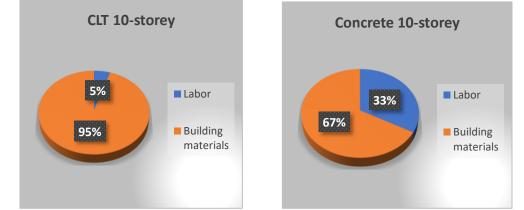
Figure 5. construction costs breakdown for a 10-storey building CLT vs. Concrete
