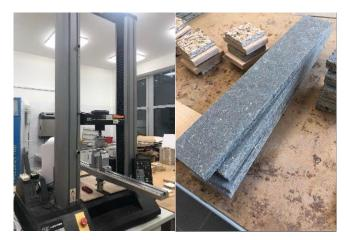
Fig.1: INSTRON IN5566 bending machine (a), specimens (b)
