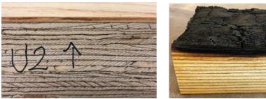
a) before fire test b) after fire test Figure 1: LVL specimen with F1-treated surface veneer
