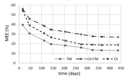
Figure 1. Moisture excluding efficiency of treated beech samples during exposition above water level (OI – oil impregnated, TM – thermally modified at 200 °C, OI+TM – combined process)
