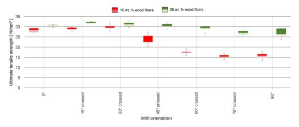
Figure 3: The behavior of the ultimate tensile strength as a function of the wood/PLA composite (composite #1 or composite #2) used and the infill orientation applied.
