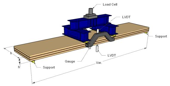
Figure 1. Bending test setup.
