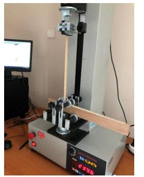
Figure 1.a. MDF edge banding test started
