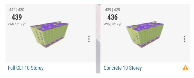
Figure 6. Energy use intensity simulation of the 2 alternatives of the 10-storey building
