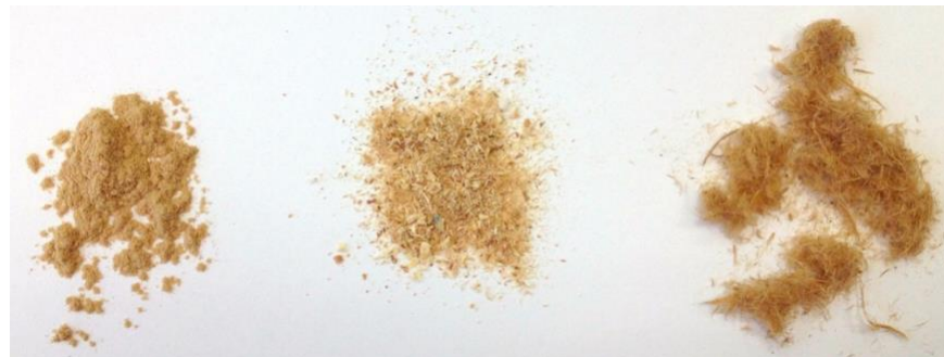
Figure 1. Image of wood flour (a.), microparticles (b.) and fibers (actually fiber bundles) (c.)
