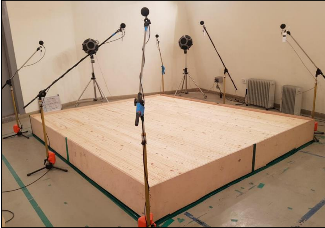
Fig.3 The test specimen installed (Test of sound absorption class)
