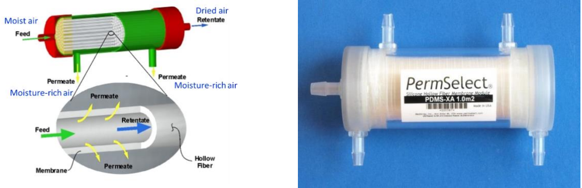
Figure 1. Exploded view of basic hollow fiber membrane (Montoya, 2010).
