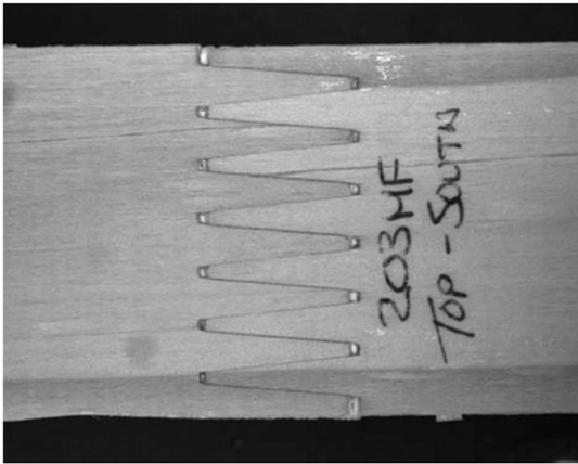
Figure 1. Representative finger joint made in the laboratory.
