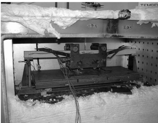
Figure 4. Sample and loading device in the oven. To load the specimen, the lever arms were brought down to rise to steel plates and apply a bending stress of 10 MPa. The load was applied normal to the plane where the fingers of the finger joint were visible.
