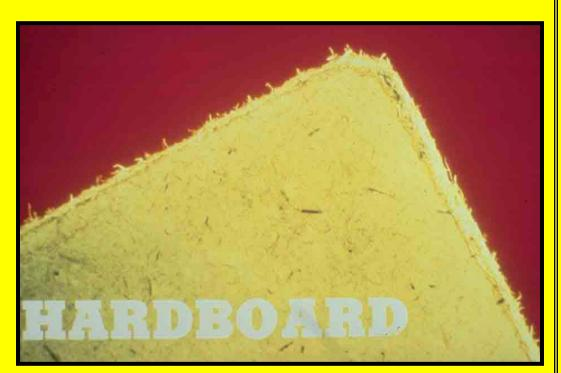
Hardboard is made from wood that has been reduced to pulp. The pulping step is similar to that employed in making newsprint. The fibers then are formed into a mat and pressed using very high temperature and pressure. The result is a hard, dense mat known as hardboard.
