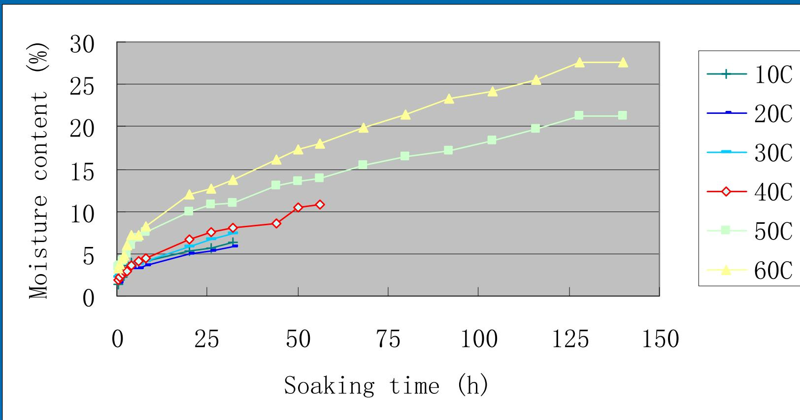
**Soaking temperature above 40 °C results in a significant higher absorbing rate**
