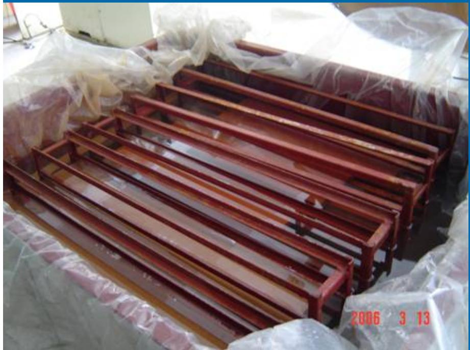
**Method: Soaking at ambient for 2days, frozen at -29°C for 2days, and thaw at ambient for 3days.**
