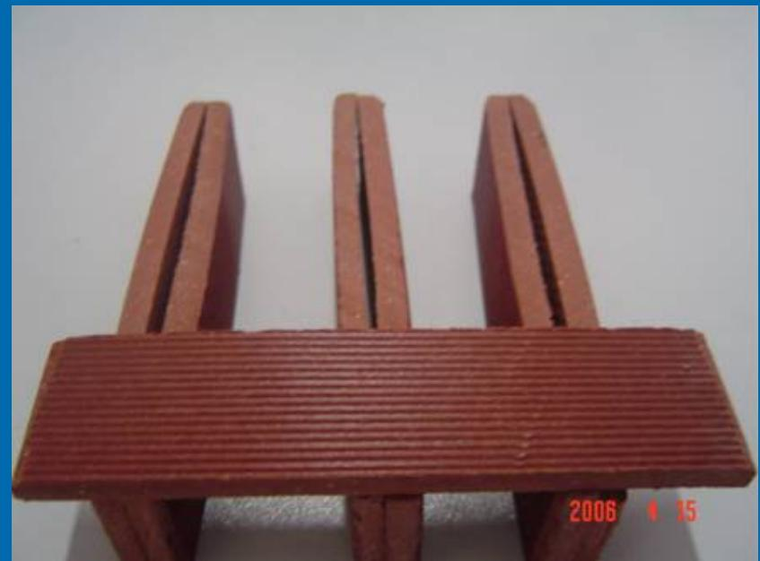
small size sample cut from surface of big sample may warp after UV accelerate weathering, which should be paid attention in service. Balance is necessary.
