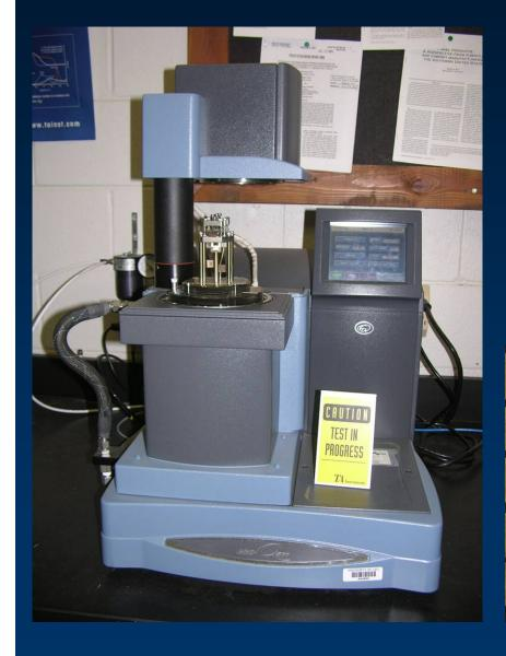
Dynamic mechanical analysis (TA Q-800) - Test runs were made in bending at a constant temperature of 25°C and a varying temperature from 25°C to 200°C with a heating rate of 2°C/min using 1 Hz frequency.
