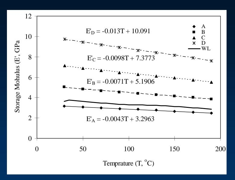
For every 10 degree of temperature increase,  $E'_{A}$ ,  $E'_{B}$ ,  $E'_{C}$ , and  $E'_{D}$  decreased by about 40, 70, 100, and 130 MPa, respectively.
