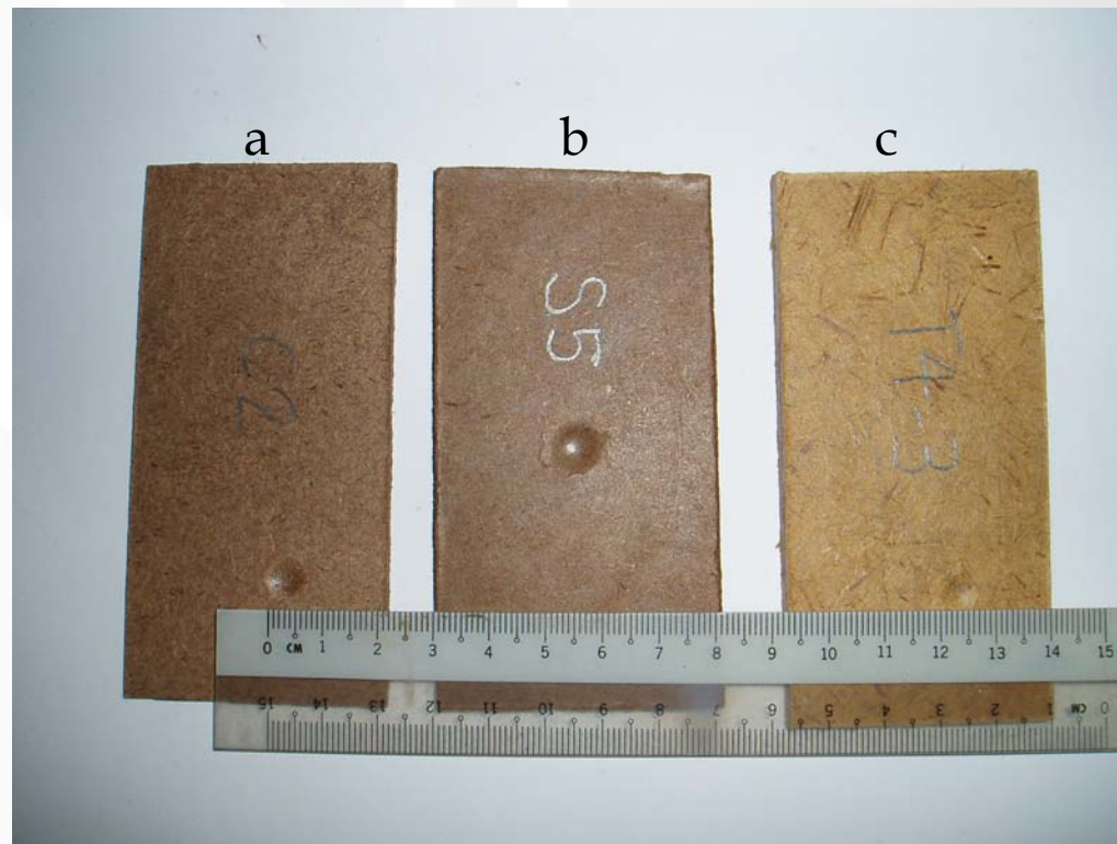
(a) Small dent resulted in commercial test sample, (b) big dent of bamboo steam pre-treated, and (c) Indistinguishable dent on NaOH pre-treated bamboo hardboard
