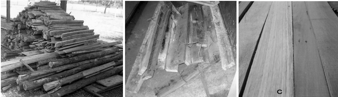
Figure 1. Various types of wood wastes collected (left) and visual aspect of wood strips for blockboard production (center); and after planning (right). Photos: author.
