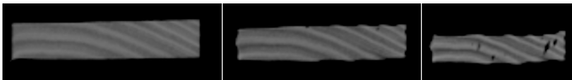
Figure 4: Sequence of the same specimens. Left: beginning of the drying. Center: collapse is visible at the surface of the specimens before any checking. Right: internal checking is visible well after the collapse.
