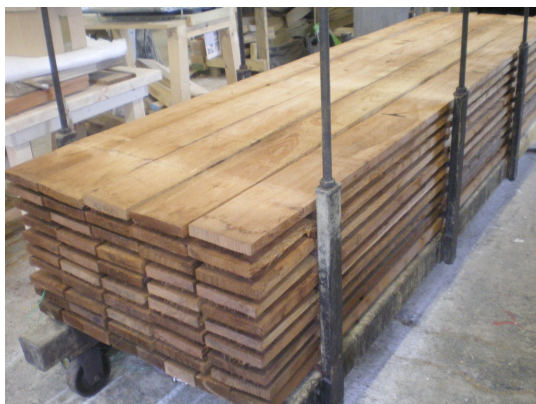
Figure 3. a) Unloading mild thermally treated larch from the scale up treatment kiln. d) Planks were successfully laminated together and machined in a 4-head cutter. Photo credit Morwenna Spear.
