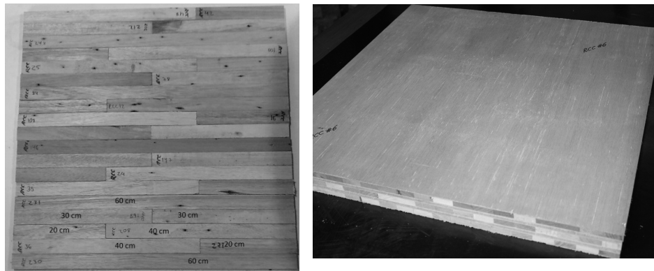
Figure 2. Core panel of 600x600 mm with 600, 400, 300 and 200 mm long wood strips (left) and blockboard assembled (right). Photos: author.
