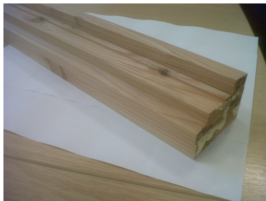
Figure 3. a) Unloading mild thermally treated larch from the scale up treatment kiln. d) Planks were successfully laminated together and machined in a 4-head cutter. Photo credit Morwenna Spear.
