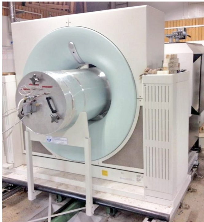
Figure 1: Drying kiln and CT-scanner. The specimen is located in the metal tube that fits within the void of the scanner.
