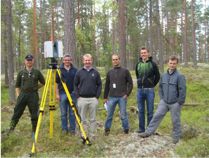
Figure 1. 3D-laser scanner acquiring data from a Scots pine stand in eastern Norway surrounded by members of the BALABU project team. The BALABU (Bakkemontert laser som verktøy for bedre utnyttelse av skogressursene) project is investigating TLS based inventory methodology in forestry.
