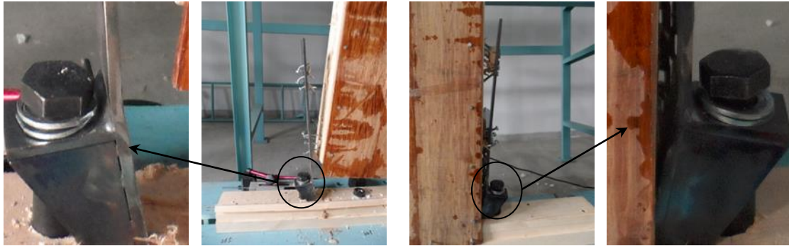
c. Diagonal of vibration exciter under cyclic load d. Lower of vibration exciter under cyclic load Fig. 6. Damage at hold-downs
