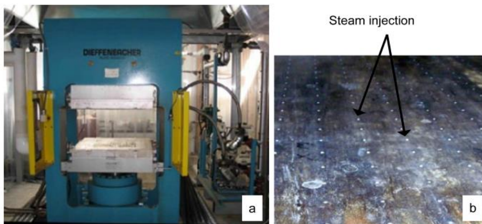
Figure 1. Steam injection hot press used for the densification treatment. a) 862 mm x 862 mm hot press, b) Press platen with steam injection holes.
