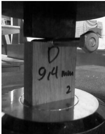
Figure 3. Typical test setup for evaluating dowel bearing strength of wood (Clemen (2013)).
