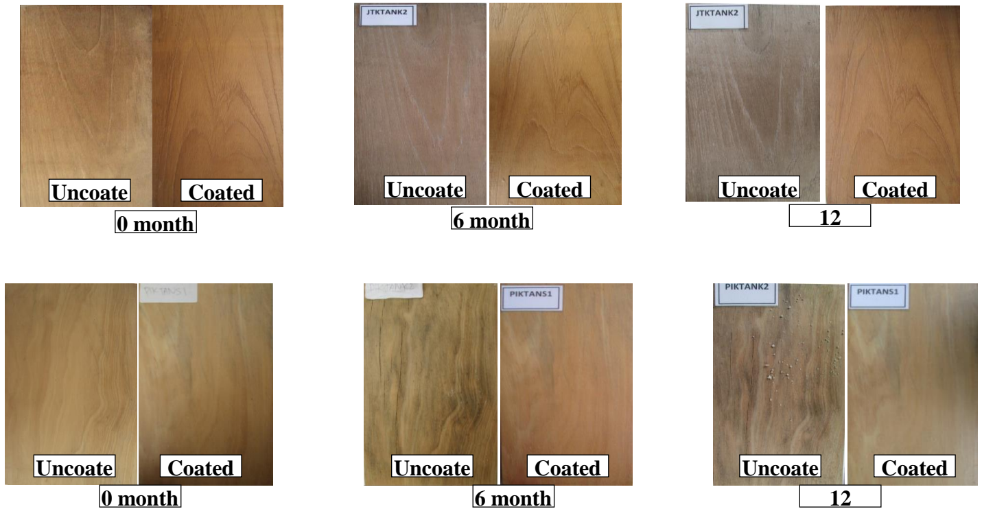
Figure 3. Uncoated and coated flat sawn teak and pine wood after one year weather exposure
