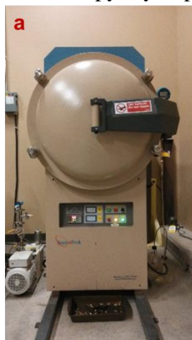
Figure 1. A box furnace (a) and (b) the internal pressure and temperature as a function of time in three pyrolysis periods: I) ramping of 10°C/min; II) dwelling for 10h; III) controlled cooling of 10°C/min and then self-cooling to room temperature.
