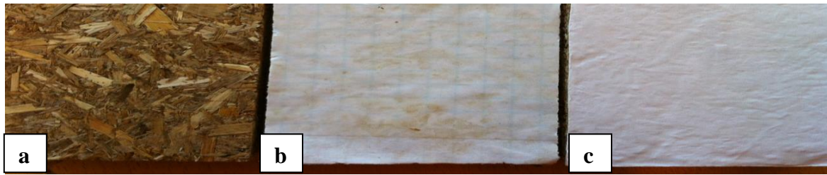
Figure 3: Particleboards manufactured out of reed canary grass glued with an acrylic adhesive a) without surface treatment, b) with lamination, and c) with paper coating
