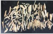
Commercial OSB strands typical of those used in a three layer panel
