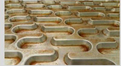
Patented, bi-directional corrugated mold
