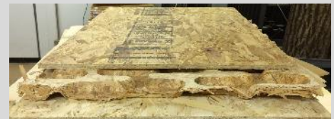
Strong axis of 9.5 mm nominal thickness (3/8 in.) 24/0 Span-Rated OSB facings oriented parallel to core length direction
