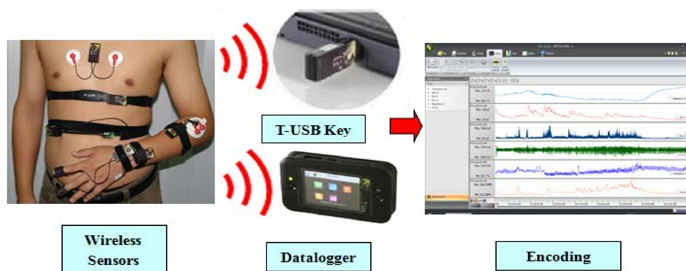
Fig. 4. CAPTIV behavior synchronous analysis diagram
