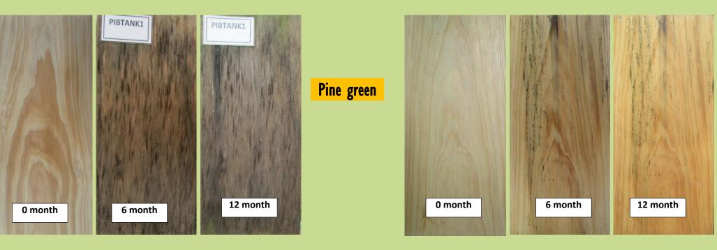
One year outdoor exposure caused mainly aesthetical changes for films of the Ultran Politur and Sayerlack. The color changes of the uncoated pine, teak, and kamper woods were prominent than that of their coated woods. Coating degradation gradually became more pronounced during the exposure. The coating films on pine after one year presented light checking that resulted in the growth of blue stains. However there were no significant checking on the film of teak and kamper.
