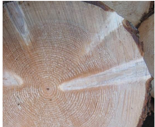
Fig. 6 Transfer zone between clear wood and knot wood
