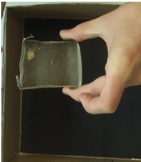
Fig. 1 Spreading and separating fibres onto a black background
