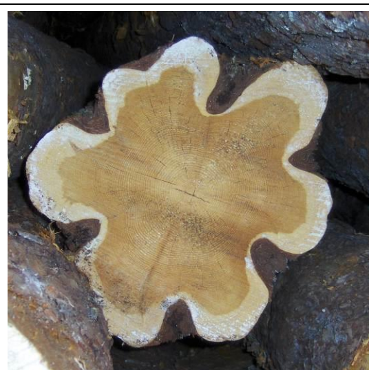
Fig. 5 Severe out-of-roundness is found near the stem base, and more in pine (picture) than spruce
