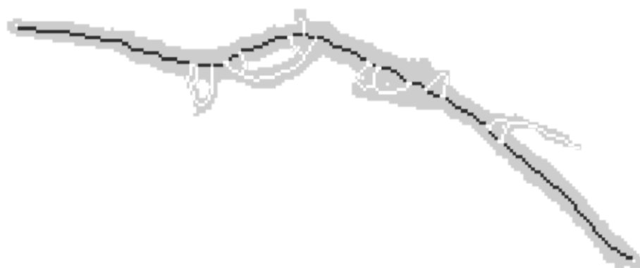
Fig. 2 Curved wooden fibre (grey) with calculated medial axis for determining the actual fibre length (black line) and length of branchings (white)
