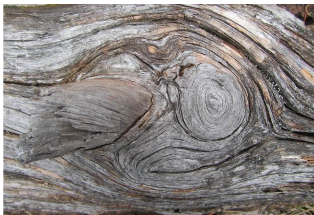
Fig. 7 a. Some trees develop ‘udder branches’ (left) b. Complex grain whirls in the transfer zone surrounding the knots (right)
