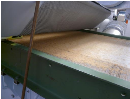
Figure 20: Airlaid head and forming sieve with well distributed fibres.
