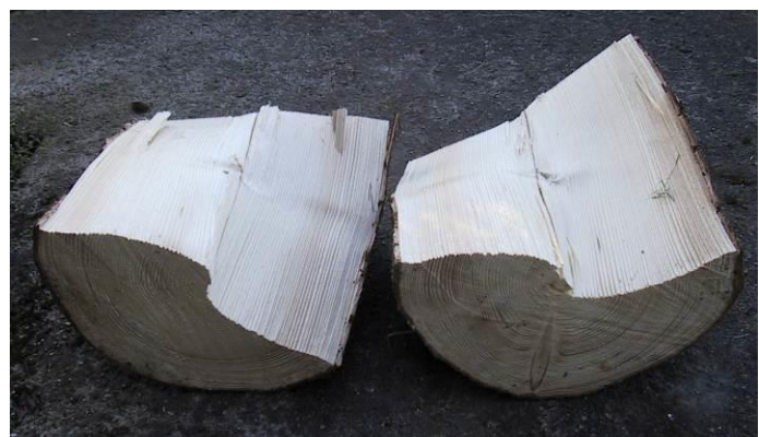
Fig. 2 Spruce opened with the split-disk method. GA changes rapidly in the juvenile wood, and subsequently linearly with distance from pith.
