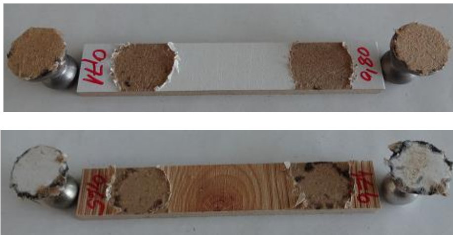
Fig. 5. The examples of images of damage arising in the researches of adhesion in the method tearing away
