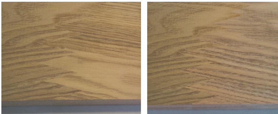
Figure 7. Appearance of the curvilinear finger jointing oak pieces
