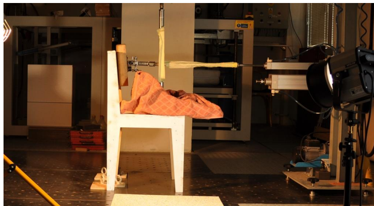
Figure 1: Chair design during testing in accredited laboratory
