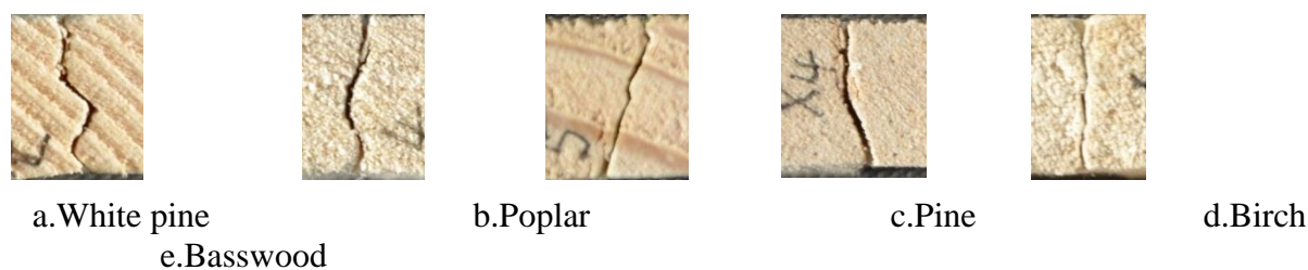
Fig. 4 Images of transvers shearing fracture profiles after thermal softening
