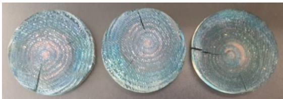
Figure 57 Penetration of wood preservatives
