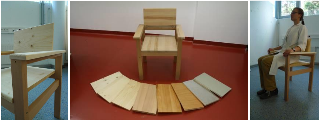
Fig. 1 Testing chair with exchangeable sets of seat, arm rests and backrests, arm rests are also usable for testing the edge radius preferences.
