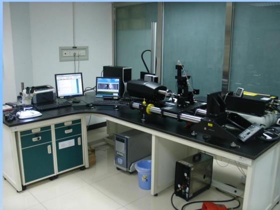
A commercial microtensile tester combined with a custom-built fiber griping system was used to measure the IFSS. This instrument was initially developed for measuring the mechanical properties of single short plant fibers, such as those found in bamboo or wood.
