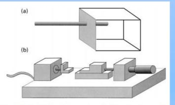
Fig. 1. (a) Single fibre pull-out specimen. (b) Schematic drawing of the loading rig.
