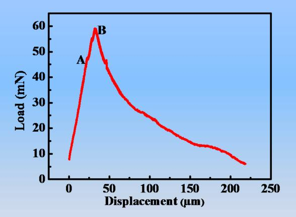
The typical single fiber pull-out curve: Load vs. displacement.
