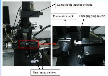
Schematic drawing showing how a single bamboo fiber pull-out test is performed
