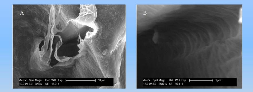
SEM micrographs: (A) the cavity left in the PP matrix after extraction of the fiber; (B) the inner surface of the cavity
