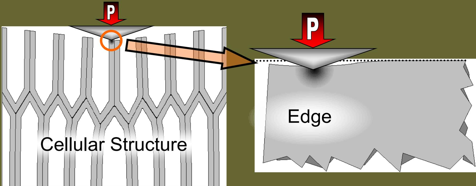
Use structural compliance method to experimentally account for specimen-scale flexing and edge effects
