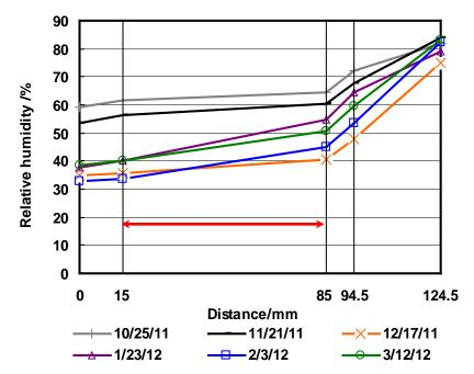
✓The maximum of relative humidity gradients was 15% from the gypsum board to the OSB sheathing.
