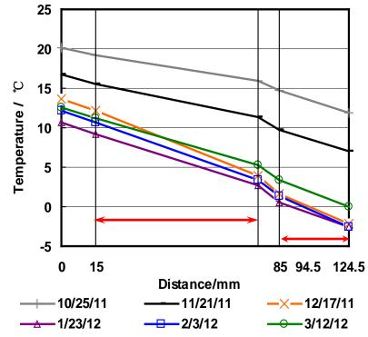
Effective function of the insulation layer and ventilation cavity.
