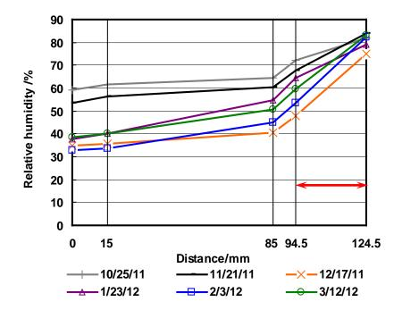
✓ Relative humidity gradients were the largest between ventilation cavity and lateral wall through the wall.
