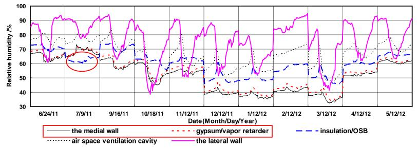
✓ Relative humidity variance of the lateral wall was from 30% to 99%, but that of the medial wall was lower, more steady and proper to live.
