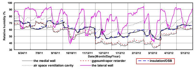
✓ Relative humidity of the interface between the insulation layer and OSB sheathing was comparatively stable, and was lower than that of inside the ventilation cavity. The difference was 7%~10%.
