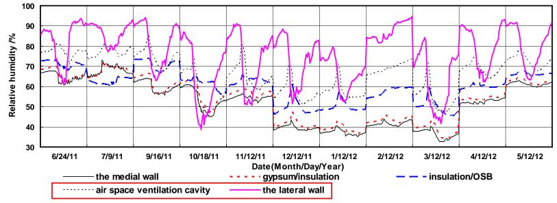
$\checkmark$  Relative humidity inside the ventilation cavity below maximum was lower than that of the lateral wall.
