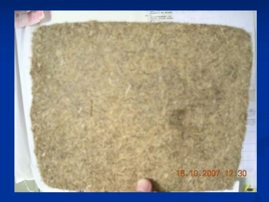
Straw fiber/HDPE powder composite by hot pressing  $(16 \times 16 \times 0.9 \text{ cm})$
