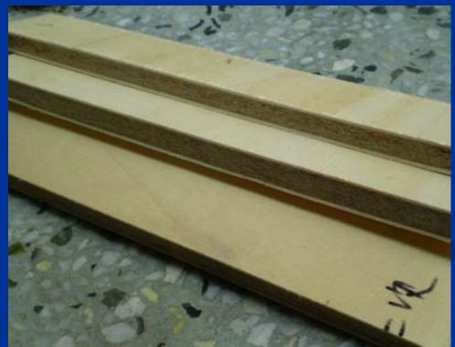
Sample treatment : Boiling/4h, Drying at  $63 \pm 3^{\circ}C/20h$ , Boiling/4h, Drying at  $63 \pm 3^{\circ}C/3h$
