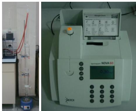
Fig. 3 Formaldehyde Emission Test Set-up (Photo: Candan)
