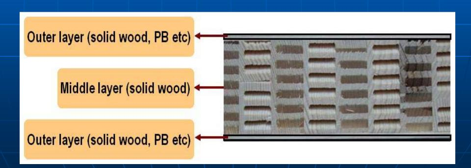
■ The middle layer of the panel consists of cross aligned boards with longitudinal kerfs, which are glued to the surface layers at an angle of 45°. The kerfs form multitude of small cells with webs inclined at an angle of
