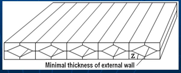
New panels need less wood in production compared to traditional cross laminated multi-layer panels. Simple geometrical calculations show that from 1 cu m of surfaced boards it is possible to produce up to 1.2 - 1.3 cu m of panels.
