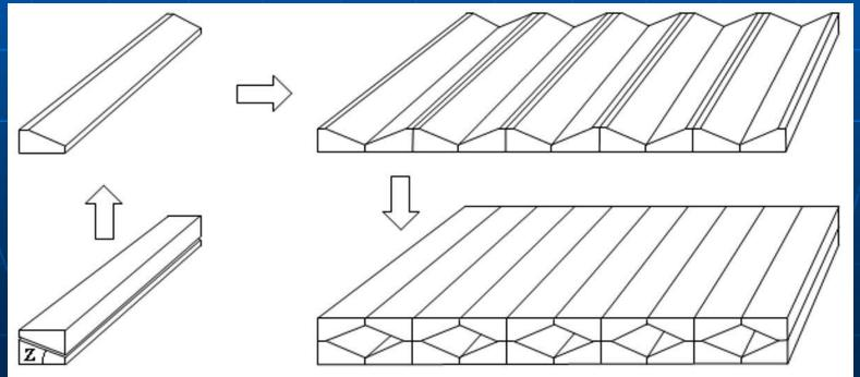
■ The angle Z depends on the cross section of the board and it defines the structure of the panel itself. The larger is the angle Z, the higher is the thickness of the panel and the lower is the minimal thickness of external wall of the panel.
