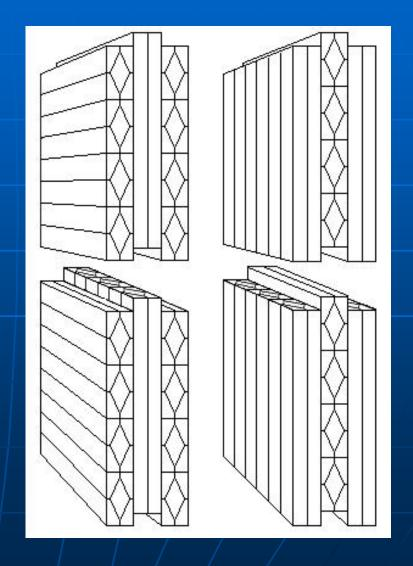
Panel appearance depends on quality of wood of external layers. When boards of 1 and 2 grades are used, surfaces can be sanded and painted. For inner layers low quality boards can be used.
