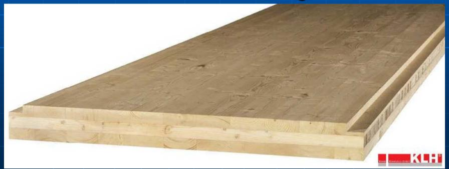
The panel thickness is determined by the end use for wall, floor, roof and smaller units for any number of custom applications. The thickness of elements is from 60 mm to 400 mm in dimensions of up to 4.80 m x 20 m.
