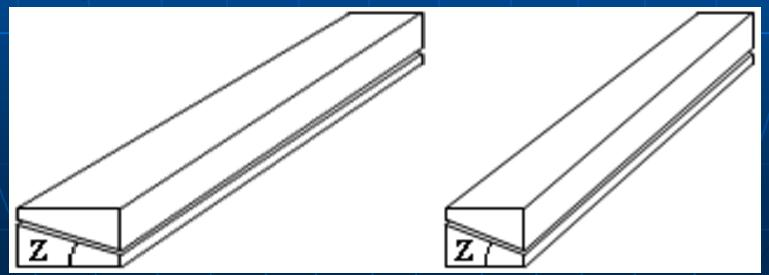
• Minimal thickness determines to a great extent the stiffness and other mechanical properties of the panel. Outer layers of panels which are exposed to external mechanical impact should have a stiffness property to withstand the impact. To accommodate that property the angle Z should be smaller. For internal layers
