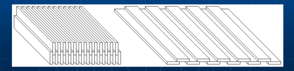
■ Fibers in the strips of adjacent layers are differently oriented, but the same angle is maintained in relation to one of the axes of the unit. For symmetry of the structure this angle should be at 45°. Slight deviation is allowed.
