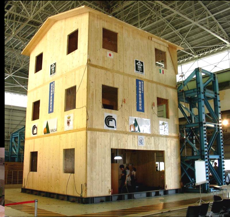
Shaking Table Test on a full- scale 7mx7mx10m of height 3 storeys X-Lam building
