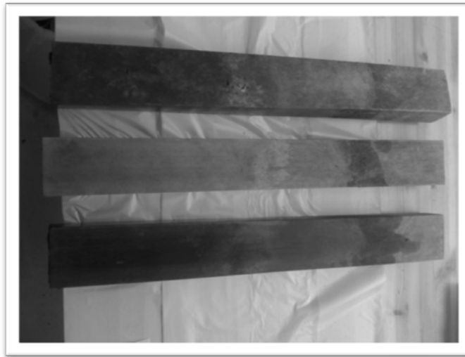
Figure 5. WPCs from in ground field tests showing white rot fungi attacked on samples with untreated wood after five years exposure while the heat treated and acetylated samples showed no signs of fungal attack.
