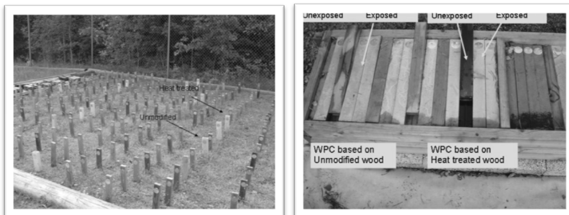
Figure 3. In ground field testing of WPCs according to EN 252 (left picture) and example of WPC test samples of unmodified and heat treated wood exposed above ground for 2 years in a so-called “Horizontal double layer test” (right picture).
