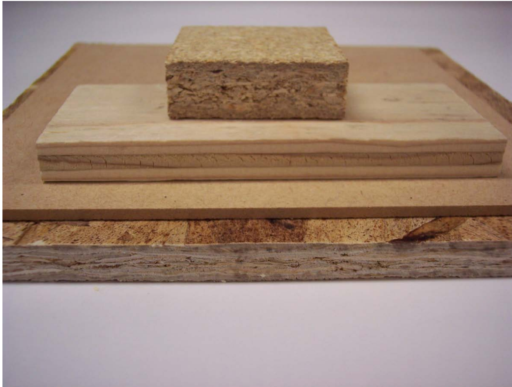
FIGURE 5 –Soy adhesive can be used commercially to make a variety of wood products, from top to bottom particleboard, plywood, fiberboard, and strandboard.
