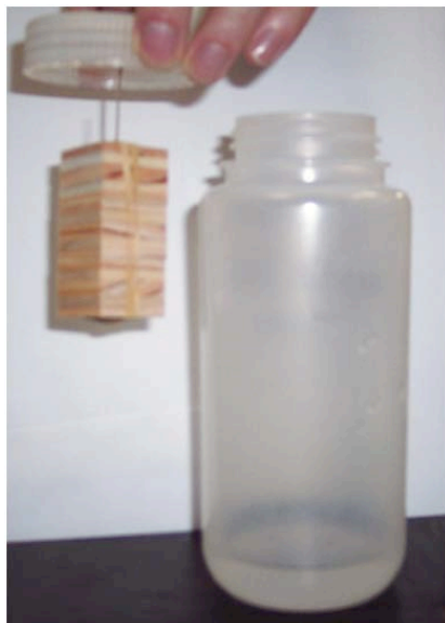
Figure 2: Sample set-up for modified EN-717-3 method
