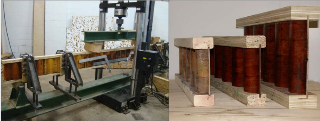
Figure 5. Set up of the third point bending tests and I joist prototypes with corrugated veneer web panels.
