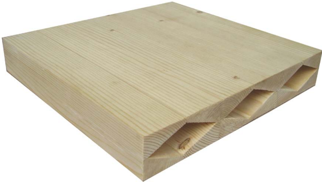
Figure 3. Lightweight solid wood panel.
