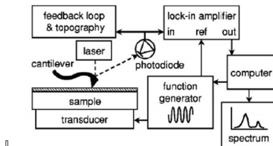
Fig 1. Schematic representation of AFAM apparatus (Hurley et al. 2003)
