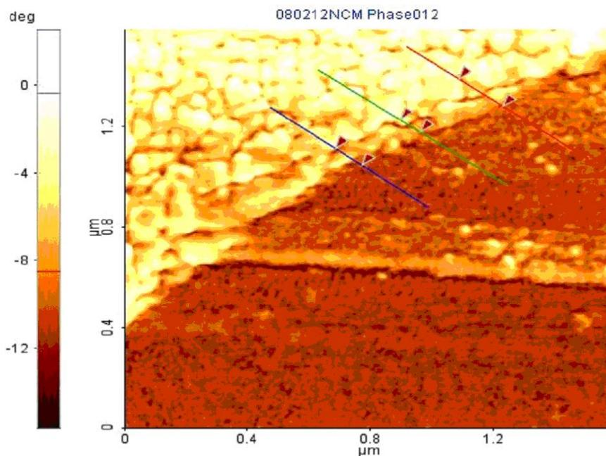
*Fig 4. Phase image of PP/10% MAPP composite*
