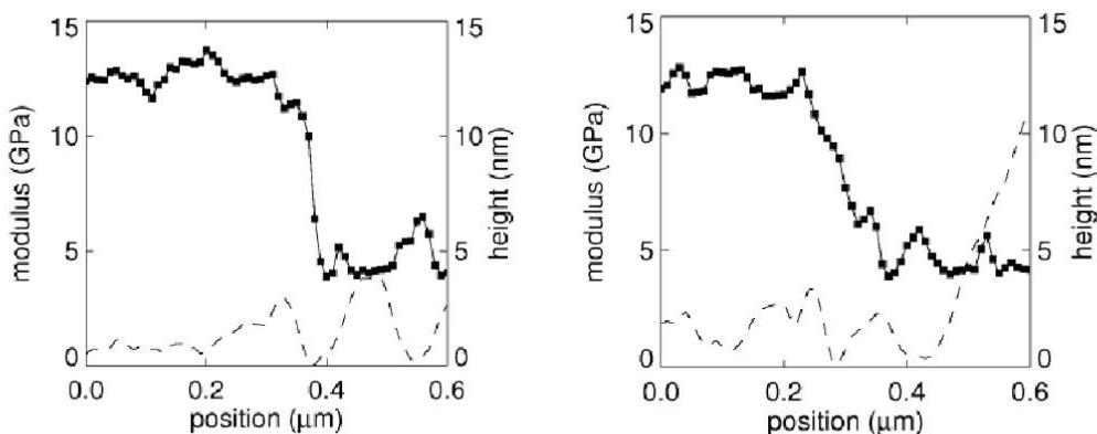
Fig 3. Variation of modulus (solid line) and topography (dashed line) across interphase region between the fiber and PP matrix. Left: upper dashed line in the topography image of Fig 2. Right: lower dashed line in Fig 2.
