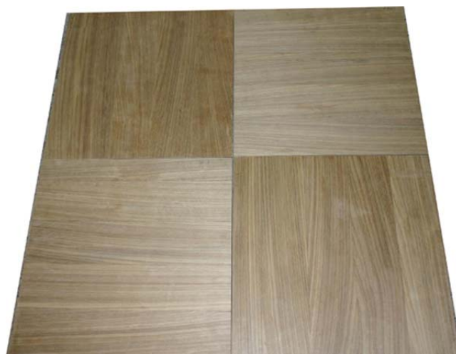
Fig. 1. CBPB flooring assembly with wood of tauari as finishing
