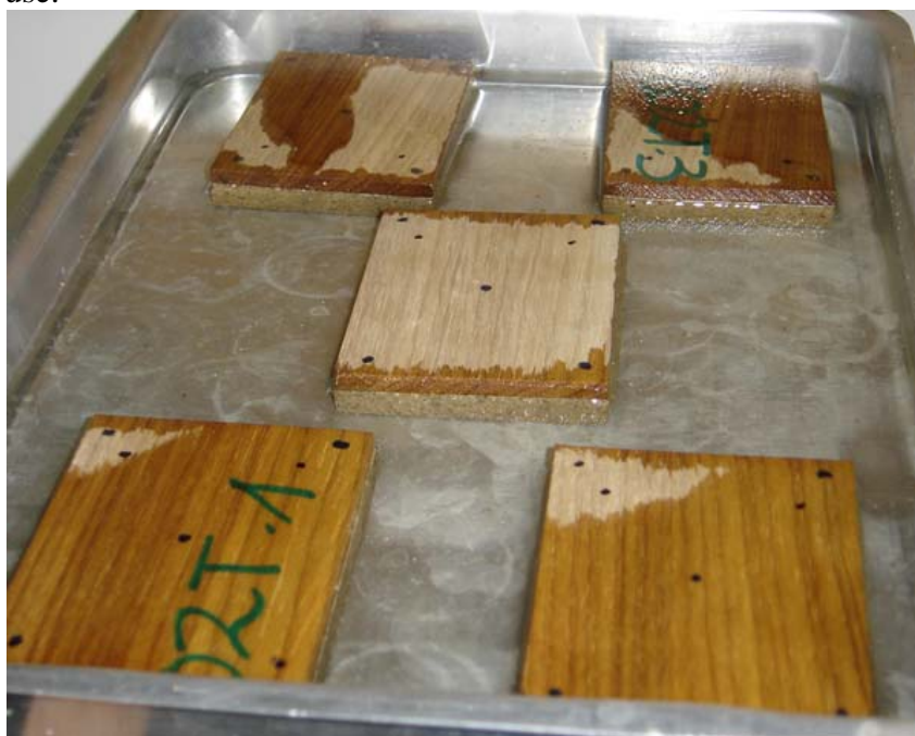
Fig. 2. Samples of CBPB flooring in the test of thickness swelling and water absorption.
