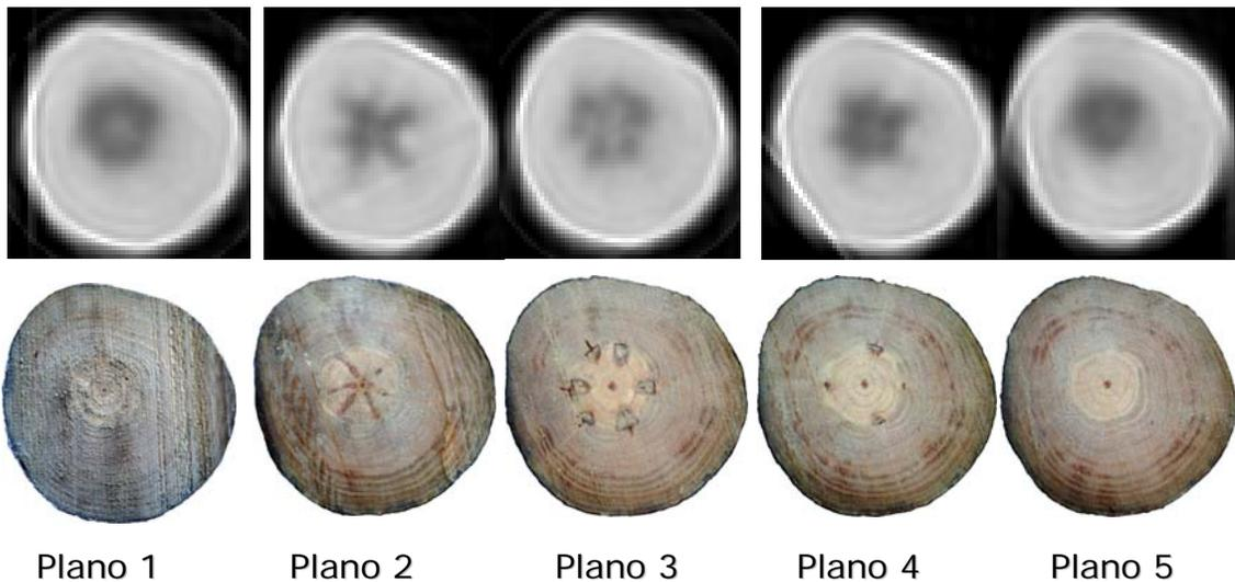
**Figure 10. Tomographic construction of irradiated planes**
