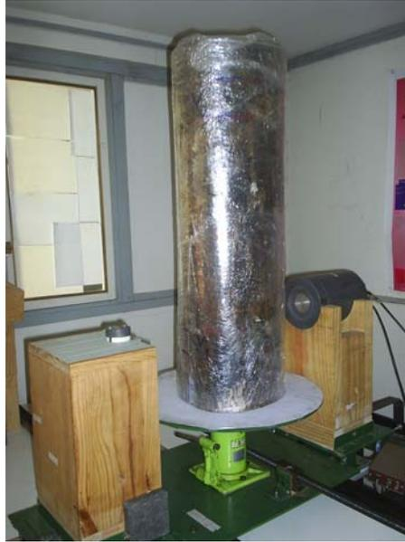
Figure 4. Log in the set of irradiation.
