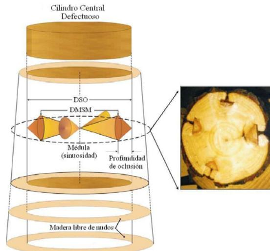
Figure 1. Defective central cylinder
