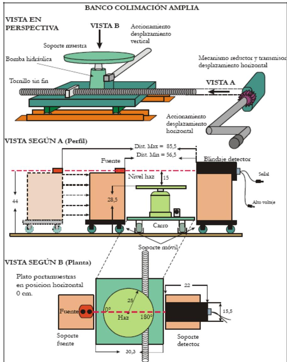
**Figure 2. Set of irradiation test**
