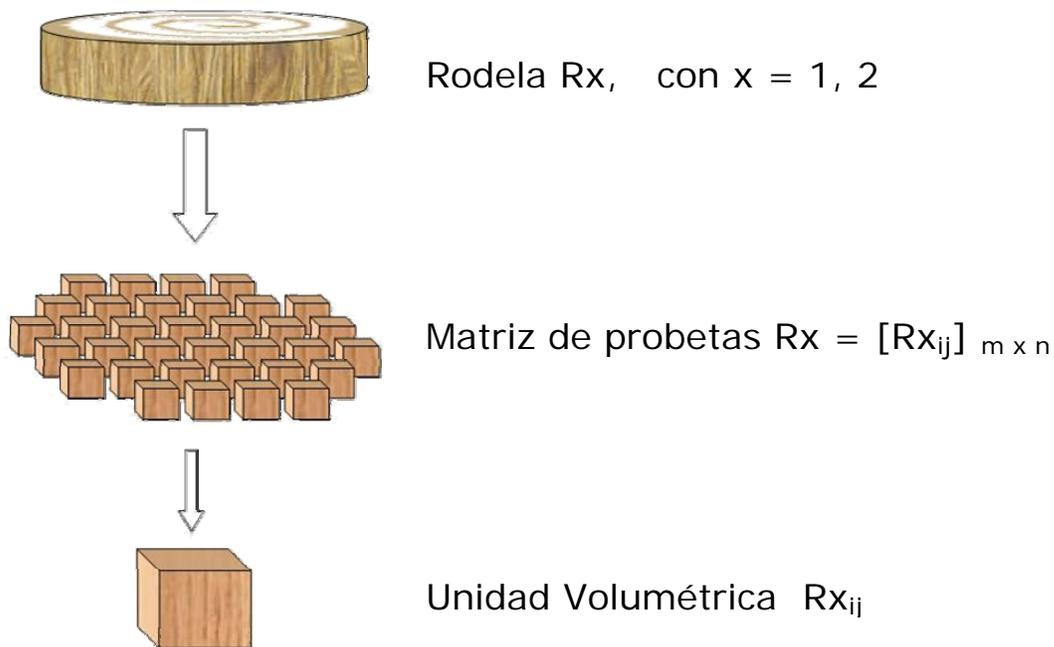
**Figure 3. Obtaining of specimens for determination of the density**
