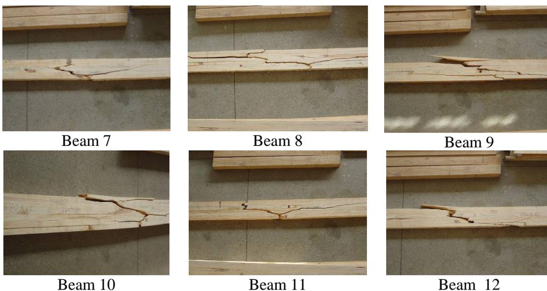
Figure 5 – Failure detail of beams with 6 lam
