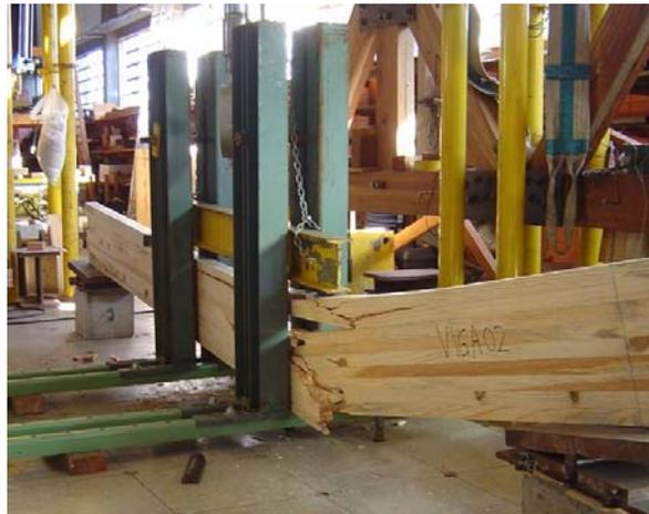
Figura 3 – Failure of beam 2
