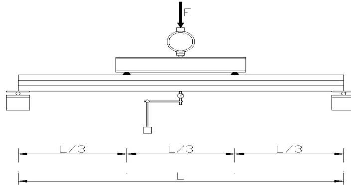
Figure 2 – Test arrangement
