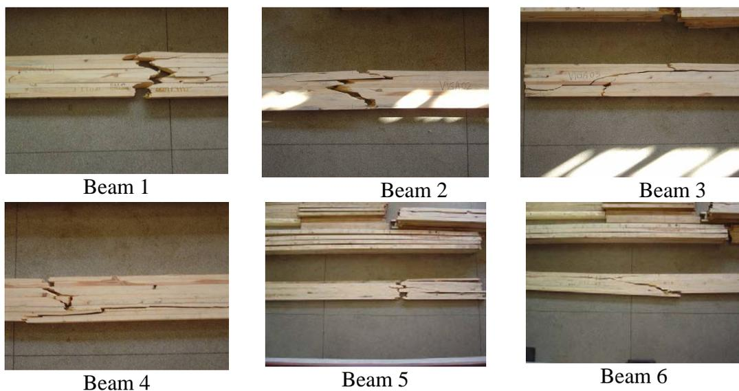
Figure 4 – Failure detail of beams with 9 lam
