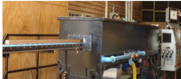
Figure 3. Extrusion of profiles for door leaves using a cone-shaped double-screw extruder (Milacron TC 35).
