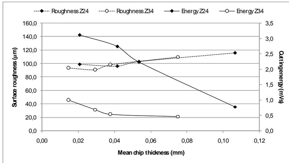
Figure 9 Relationship between surface roughness (Rz) – cutting energy depending on mean chip thickness and type of saw for 18 mm board
