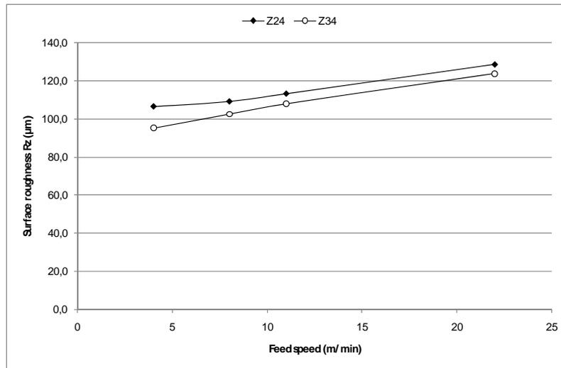
Figure 3 Surface roughness behaviors by feed speed for both saws
