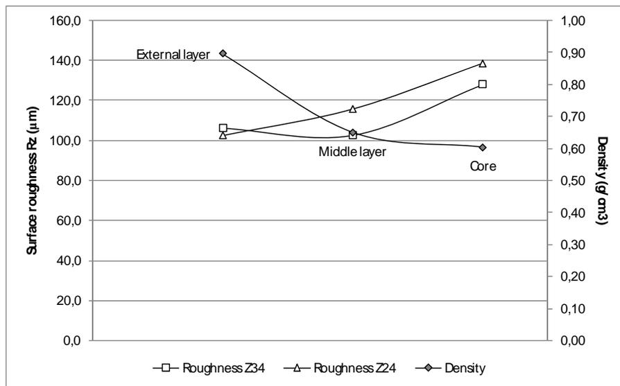
Figure 4 Surface roughness in 9 mm board by saw and density layer
