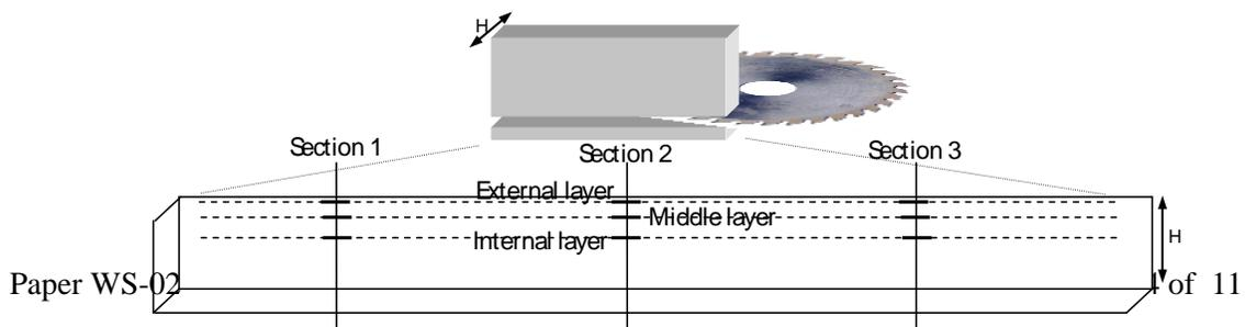
Figure 1 Outline for measuring surface roughness on 9 mm thick board.
