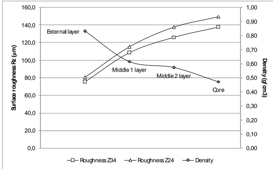
Figure 5 Surface roughness in 15 mm board by saw and density layer
