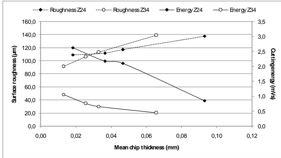
Figure 7 Relationship between surface roughness (Rz) – cutting energy depending on mean chip thickness and type of saw for 9 mm board
