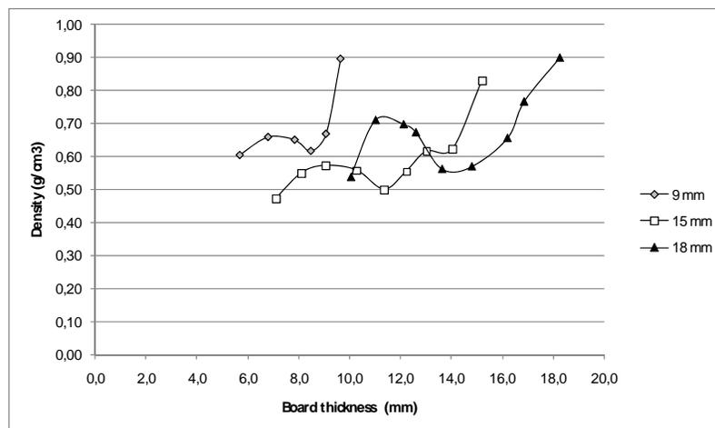
Figure 2 Density profile for studied boards
