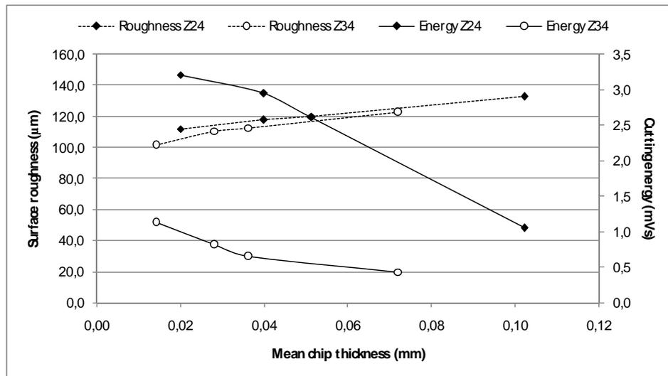
Figure 8 Relationship between surface roughness (Rz) – cutting energy depending on mean chip thickness and type of saw for 15 mm board
