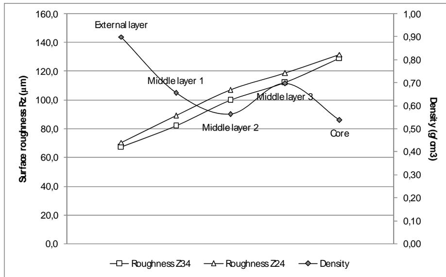
Figure 6 Surface roughness in 18 mm board by saw and density layer
