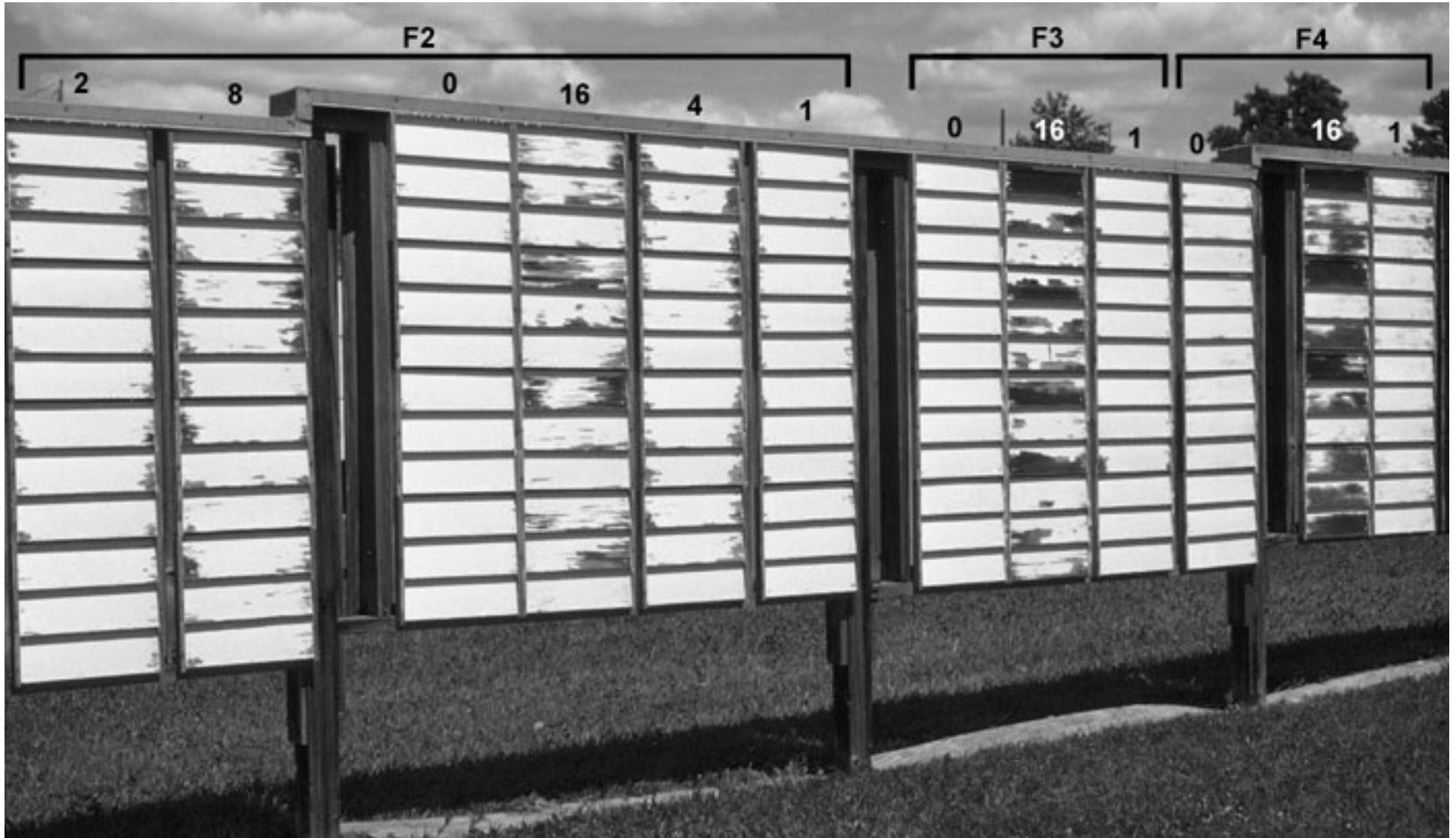
Painted panels on test fence near Madison Wisconsin after 17 years
