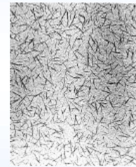
Cellulose nanocrystals 200 nm long, 10 nm wide
